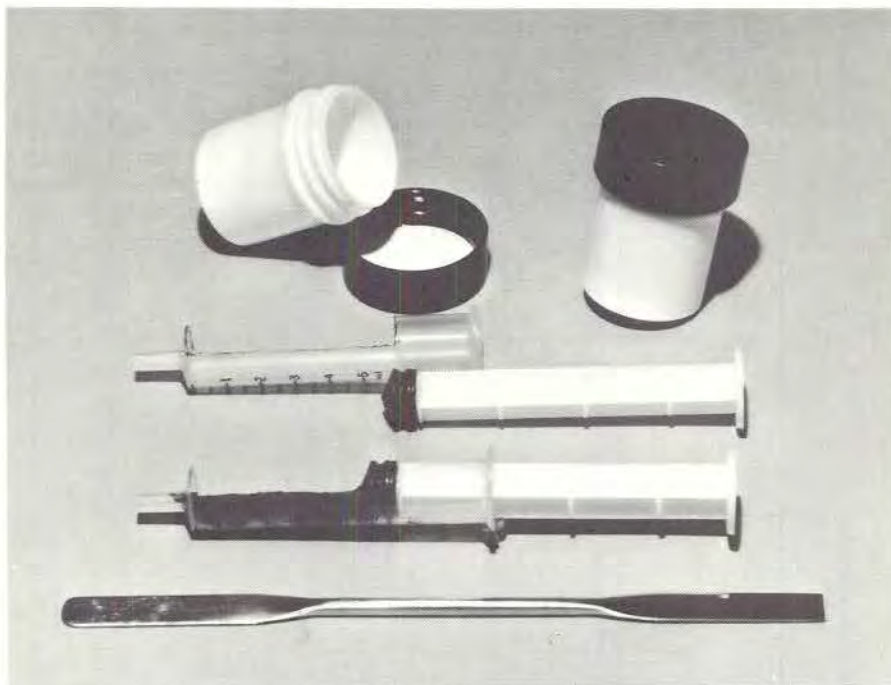
Fig. 31. Empty modified syringe, level-full syringe, plastic screw-top jars, and spatula used in determining some properties of Organic soils.
