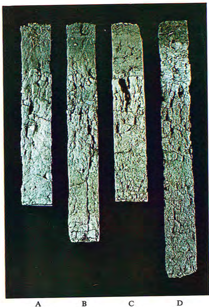
Fig. 7. Soil monoliths representative of certain Solonetzic soils: (a) Brown Solonetz, (b) Black Solonetz, (c) Brown Solod, and (d) Gray Solod.
